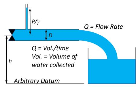
Question: How do you find the mean velocity in a pipe given the flow rate (Q)?
