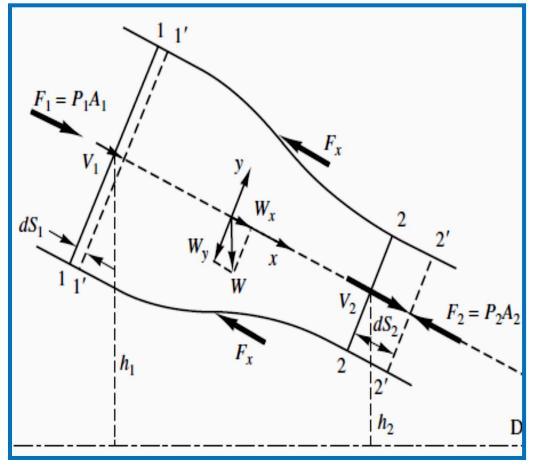
Mass flux in = Mass flux out  $\gamma [d(Vol_{1-1'})/dt] = \gamma [d(Vol_{2-2'})/dt]$  $\gamma A_1[d(S_1)/dt] = \gamma A_2[d(S_2)/dt]$ where S = velocity, thus  $\gamma A_1(V_1) = \gamma A_2(V_2)$  $A_1(V_1) = A_2(V_2)$ (2<sup>nd</sup> Key Equation) The continuity equation for steady,
