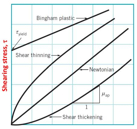
Rate of shearing strain, du/dy
