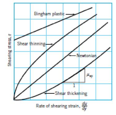
Rate of deformation is proportional to shear stress
