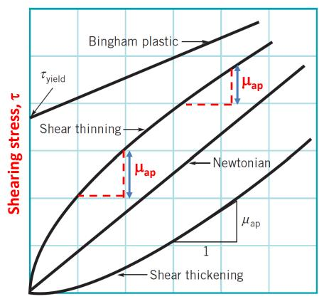
Rate of shearing strain, du/dy
