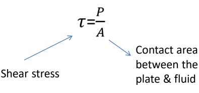
After the initial transients, upper plate moves continuously under the influence of the force (P) at a constant velocity, U
