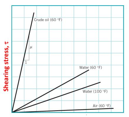
Rate of shearing strain, du/dy
