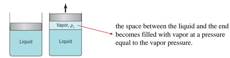
Similarly, if the end of a completely liquid-filled container is moved as shown in the figure without letting any air into the container
