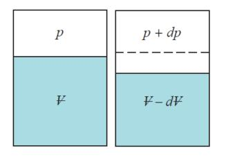
$\Delta P$  change in pressure (pressure increase)  $\Delta Vol$  change in volume (pressure increase cause the volume to decrease)
