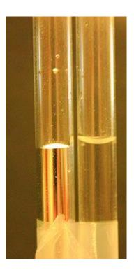
Most liquids adhere to solid surfaces. The adhesive force varies, depending on the nature of the liquid and of the solid surface.
