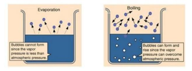
At standard atmospheric pressure, water will boil when the temperature reaches 100 °C
