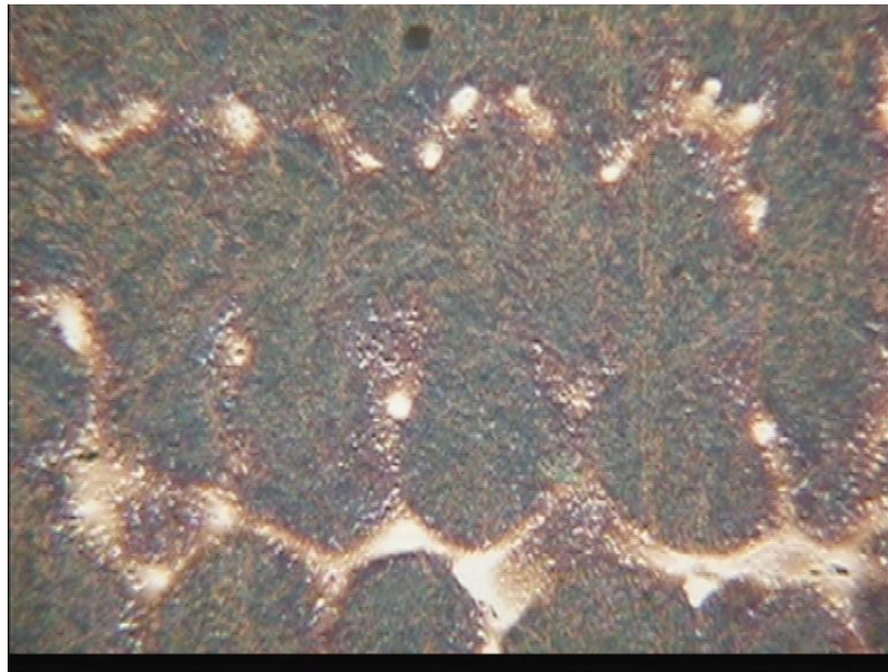
FigureV.3 Highly segregation lines between primary arms and some spot segregation points between primary arms surrounded by secondary arms (X200)
