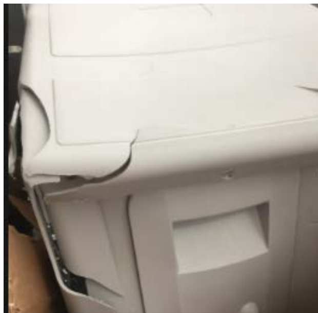
Figure 1.7 Top Cover Broken Outdoor Unit
