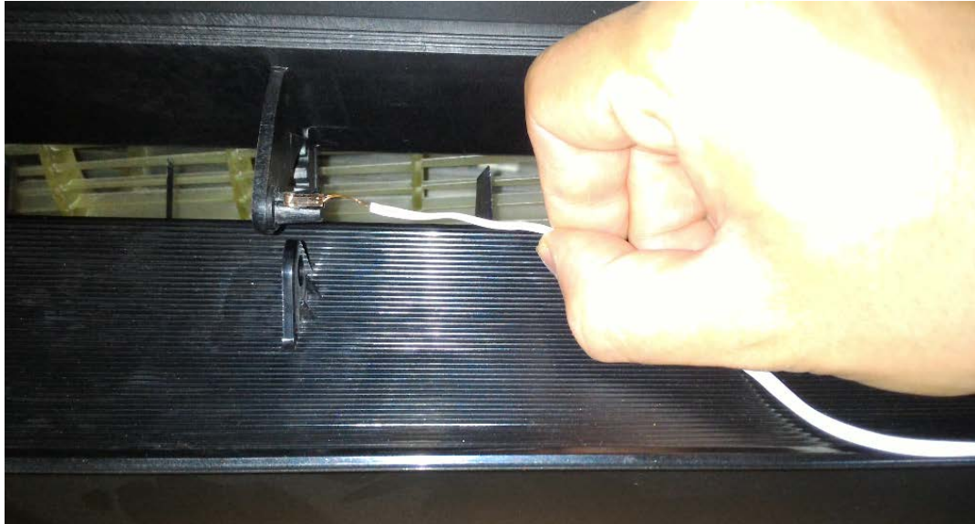
Figure 3.12 Drop Tested and Undeformed Hook of Discharge Part
