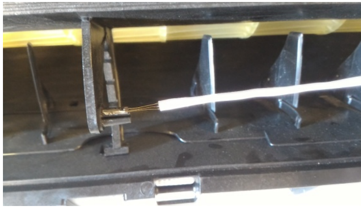
Figure 2.113 Discharge Grille Hook Strain Gauge Attachment
