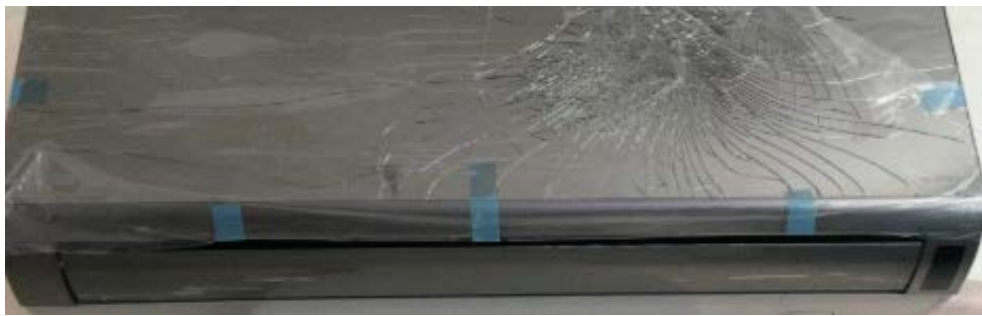
Figure 1.6 Front Glass Broken Indoor Unit
