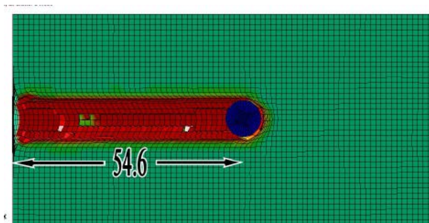
Figure 1.41 Penetration Depth for Compressed Foam [28]
