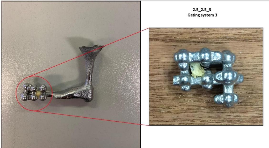
**Figure 6.24.** An illustration of the extracted 2.5\_2.5\_3 lattice structure integrated with gating system 3.
