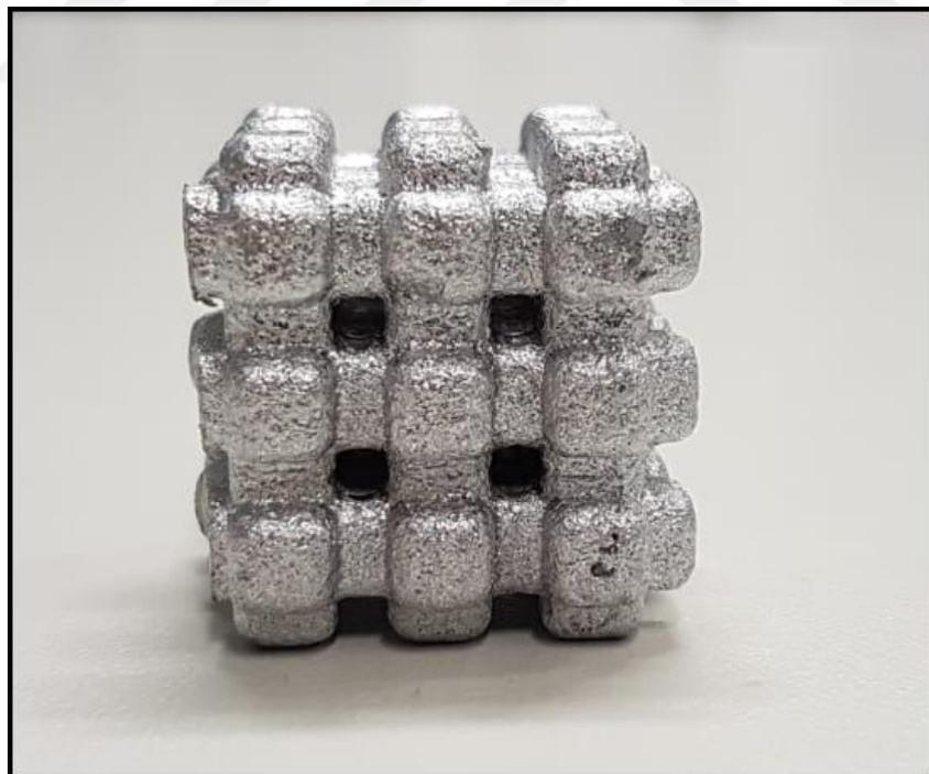
**Figure 6.32.** An image of the lattice structure of 5\_2.5\_3.
