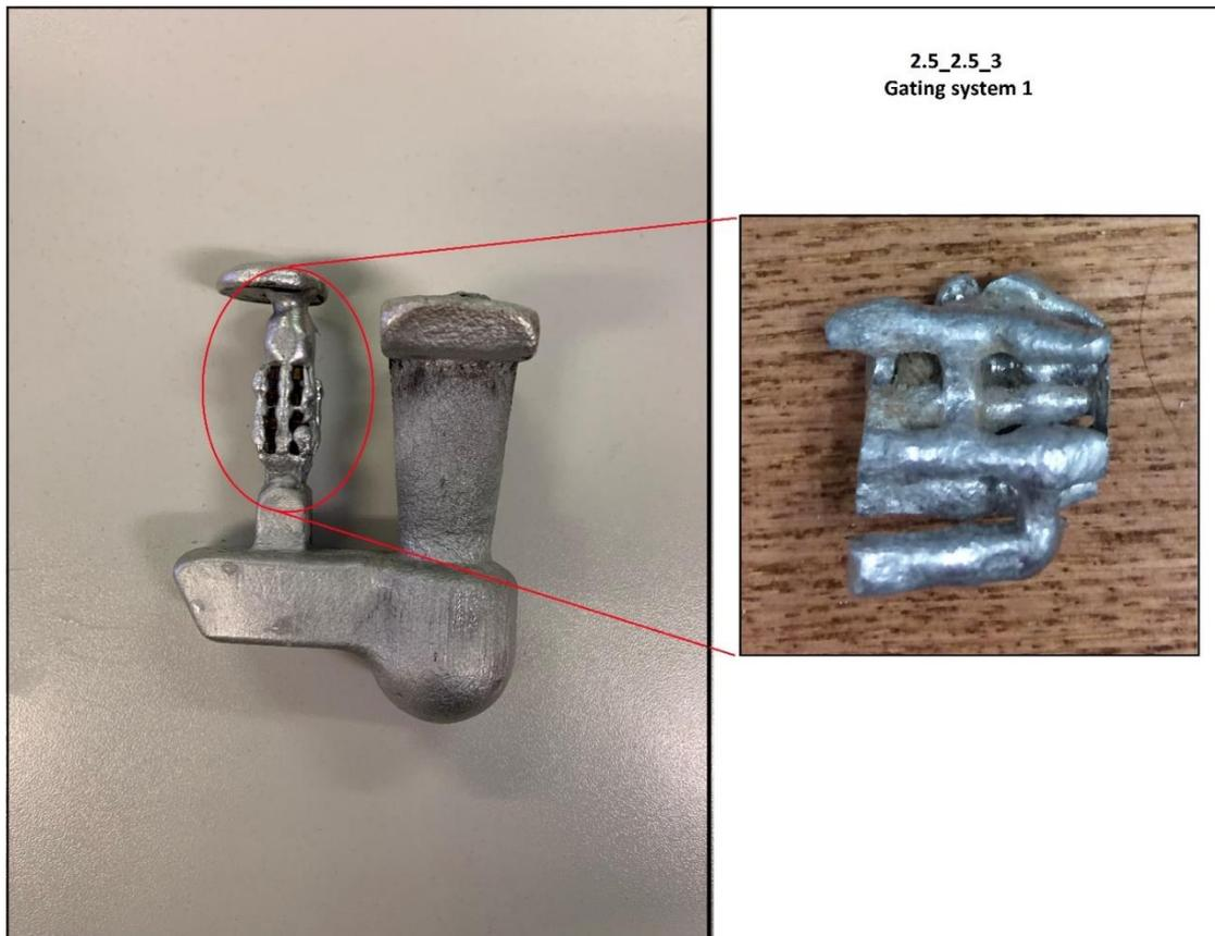
**Figure 6.26.** An illustration of the extracted 2.5\_2.5\_3 lattice structure integrated with gating system 1.
