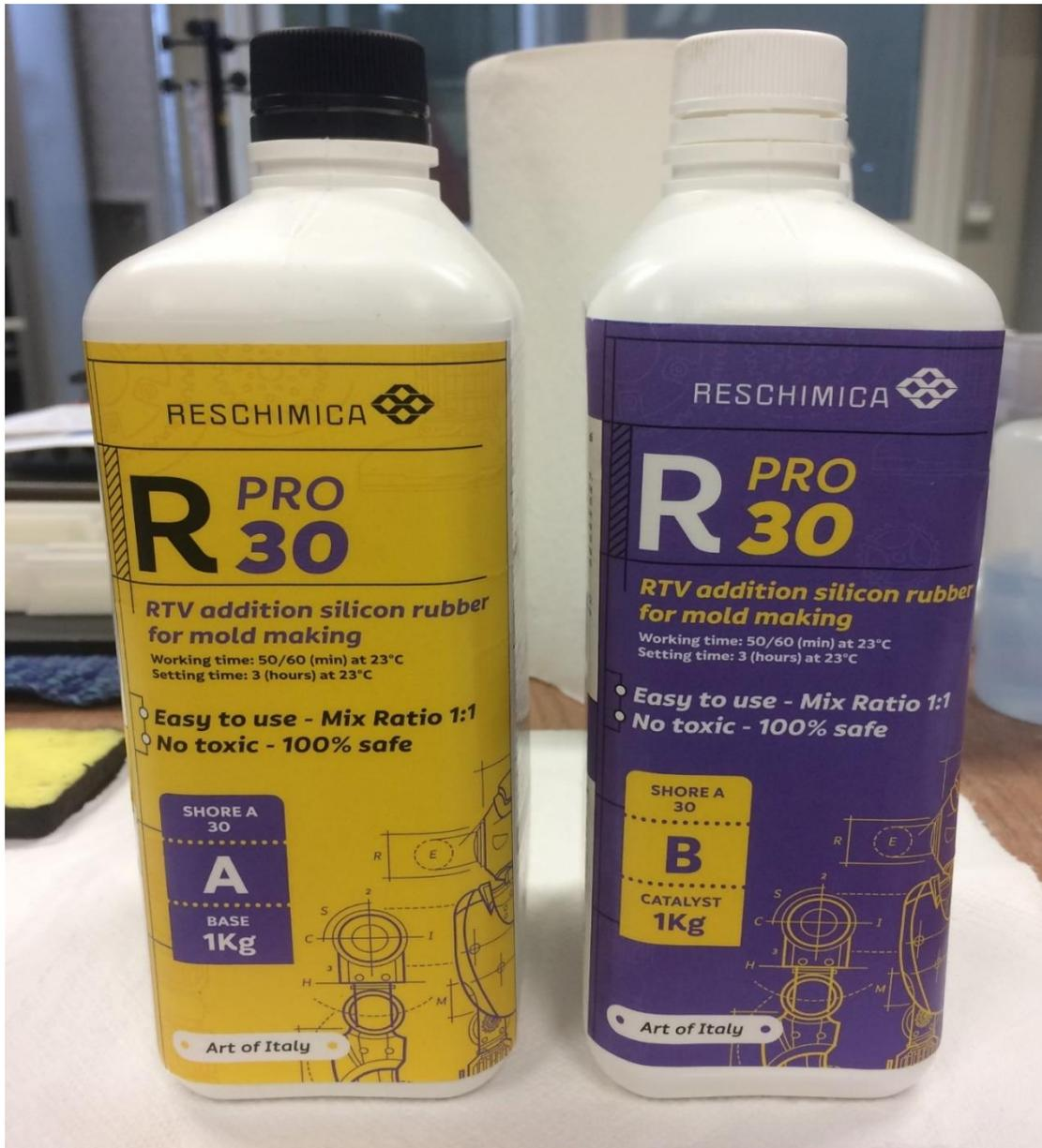
**Figure 6.2.** An illustration of the silicone rubbers of R PRO 30 A and R PRO 30 B.
