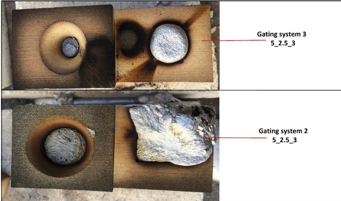
**Figure 6.15.** The illustration of the cast molds of the geometry 5\_2.5\_3 combined with gating systems 2 and 3.
