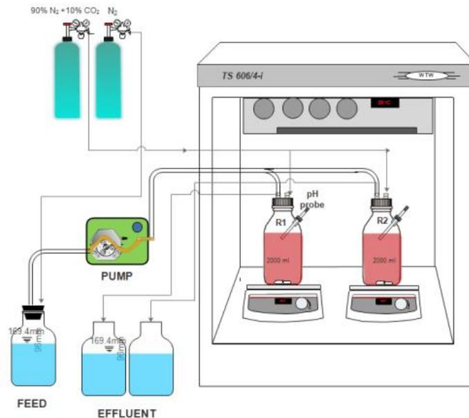
**Figure 2. 3** Schematic figure of the SBR reactors (R1: Enriched culture that was used for batch experiments, R2: Reactor that was used for investigating the Cd effect)
