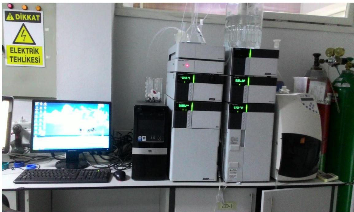
**Figure 2. 6** Shimadzu High-Pressure Liquid Chromatography with Prominence UFLC system.
