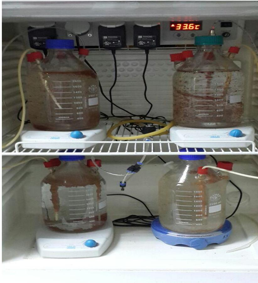
**Figure 2. 4** Experimental setups for the SBR reactors
