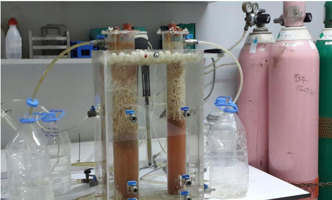
**Figure 2. 5** The experimental setup of up-flow continuous Anammox reactors
